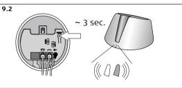
**9.2** Then press reset button on base unit for 3 seconds. Visual indicator on base unit will light constant blue
